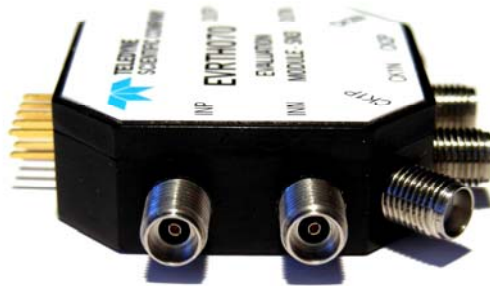
Figure 6 – Side view showing the input, K connectors
