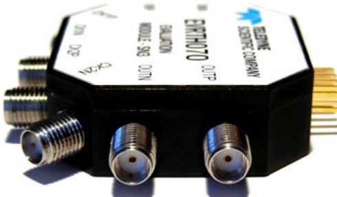
Figure 7 – Side view showing the output, SMA connectors
