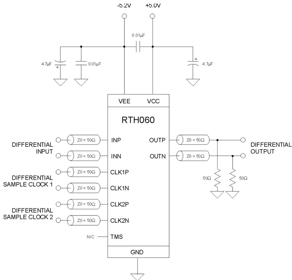
**Figure 5 - Typical interface circuit (sampled mode, connect TMS to GND for track mode)
