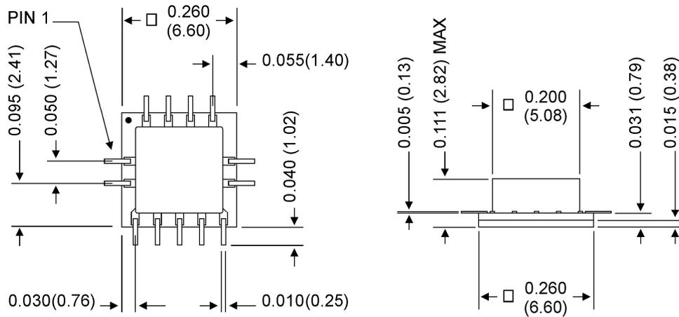
Figure 10 - RTH060-HD package outline, dimensions in inches (mm), tolerance  $\pm 0.003''$  ( $\pm 0.072\text{mm}$ ).
