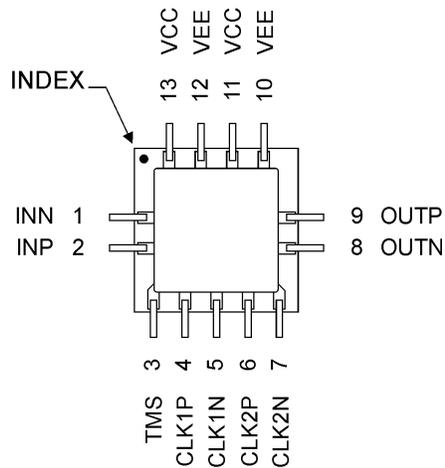
**Figure 2 - RTH060 pinout (top view) 13 lead HSD Package.**
