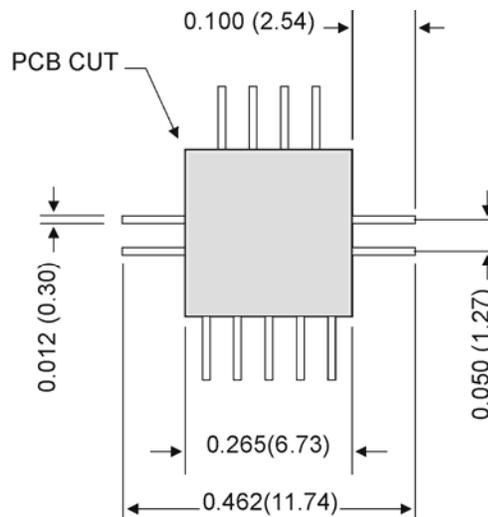
Figure 11 - RTH060-HD footprint, dimensions shown in inches (mm).
