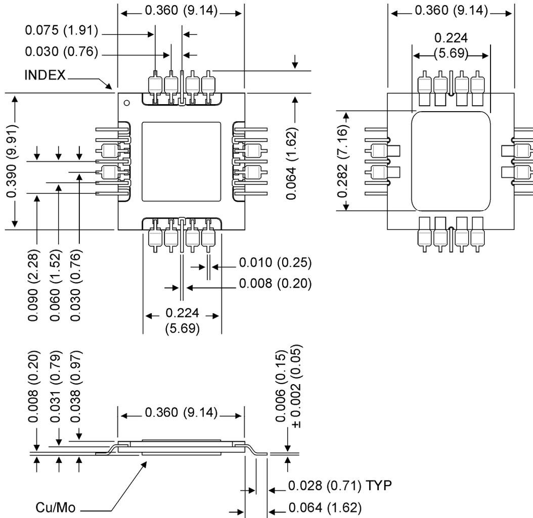
Figure 12 - RTH060-HQ package outline, dimensions in inches (mm).
