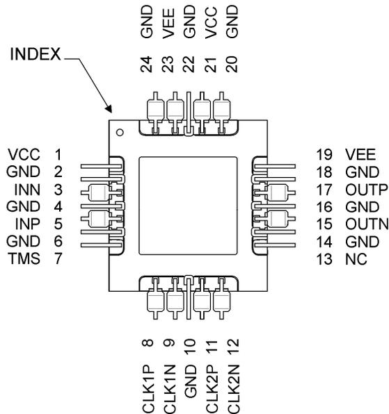
**Figure 3 - RTH060 pinout (top view) 24 lead QFP package.**
