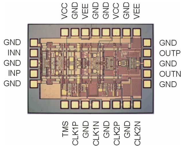
**Figure 9 - RTH060 die photo and pad arrangement; Die size: 75 x 55 x 7 mils (1.899 x 1.375 x 0.178 mm); Pad pitch: 5.91 mil (0.150 mm); Die photograph for pad placement reference only.**
