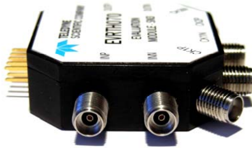
Figure 6 – Side view showing the input, K connectors
